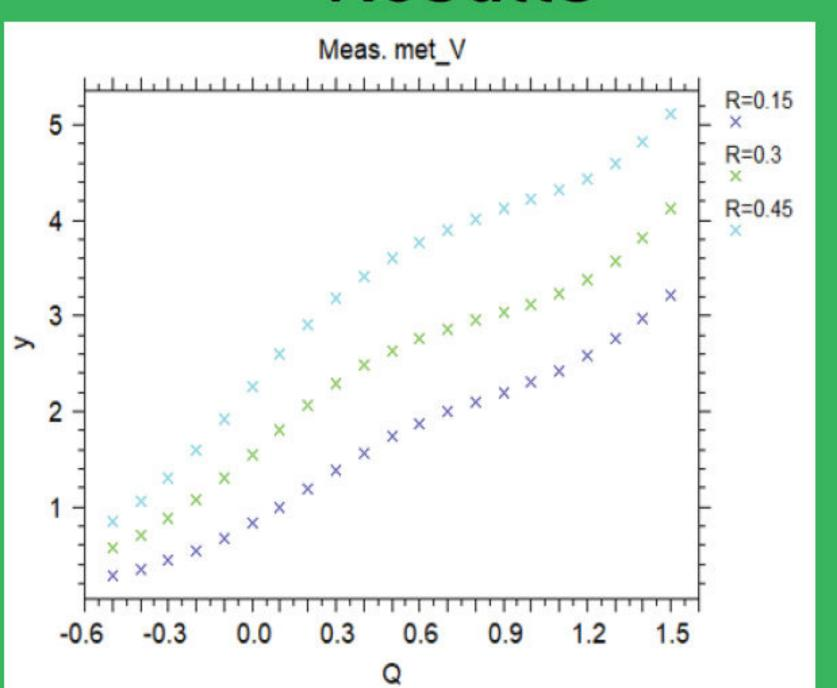
As Q increases, the wavelength decreases, meaning that a smaller wavelength corresponds to a higher V number. As the hole diameter increases, the V number increases.
